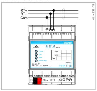
In order to terminate the RS485 network and balance the line impedance, you must enter the terminating resistor (120  $\Omega$ ), by setting ON the 1-way microswitch B.
