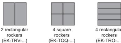
The application program allows to configure the device with ETS taking into account the number and type of rockers chosen. The three-positions rockers have central neutral position. The function carried out by the rocker depend on the configuration done with ETS. Pushing one side of a rocker (for example the upper one), the pushbutton sends on the bus a telegram for switching on, increasing the brightness of luminaires or raising the blinds, while pushing the other side (for example
